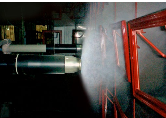
High speed bell, RPM 5,000 to 45,000 RPM, loaded
